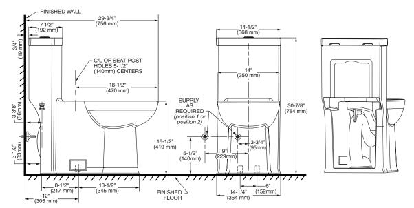
IMPORTANT: Water supply on the wall is required at 3-3/4" or 9" from centerline of the toilet (see rough-in). First suggested position is hidden behind the toilet. The geometry of the toilet gives space for this installation. The second suggested position is next to the toilet. Between these two positions, the space for the supply between wall and toilet is limited to 3-1/4". In this case, check your supply and hose dimensions.
